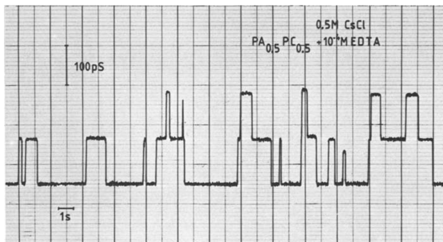
Fig. 1. Record of conductance fluctuations of gramicidin A in a 1:1 mixed membrane of PA and PC. The electrolyte contained 0.5 M CsCl and 10^{-4} \text{ M} EDTA. T = 36^\circ \text{C} , pH 6. The full bars indicate the conductance scale of the ordinate and the time scale of the abscissa, respectively. The applied membrane voltage was U = 100 \text{ mV}
